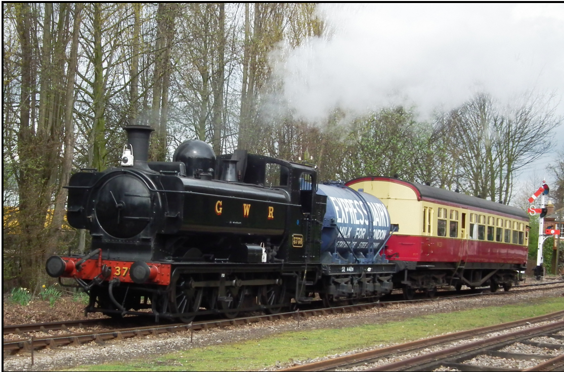
Although not actually on a preserved 'byway', 5700 Class 0-6-0T No. 3738 is seen at the Great Western Society site at Didcot on April 3 rd this year with a six-wheeled milk tanker and autococh epitomising the archetypal GWR branch line train. The Collett-designed locomotive was constructed in 1937, and was one of no less than 863 of the same Class! Photo: Peter Heath
